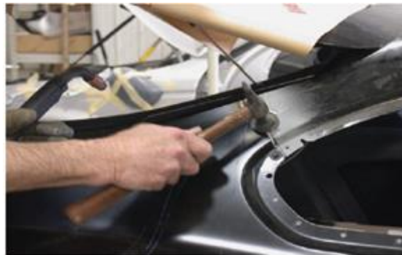
Figure 2- 21 straightening minor bumps and dents
