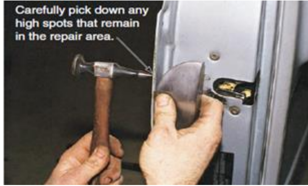
Figure 2- 31 A pointed head or pick on hammer
