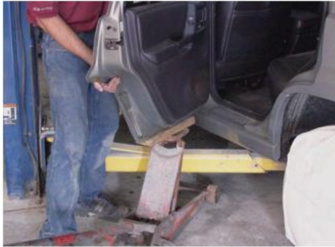
Figure 2.5. When loosening door hinge bolts, make sure the door is held so it does not fall off the jack.
