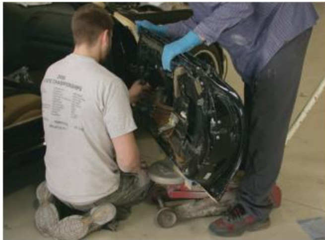
Figure 2.2B. Note how two technicians are working together to install a freshly painted door without damage.
