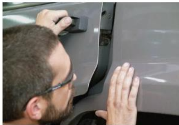
FIGURE 2.14 The first time you close the door after installation, close it slowly and softly while watching how the door fits.
