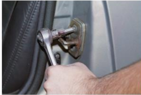
FIGURE 2.15 here the technician is using a ratchet and torx socket to install and tighten the door striker.
