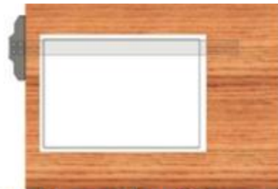
c) Align the top edge of the paper with T-square blade.
