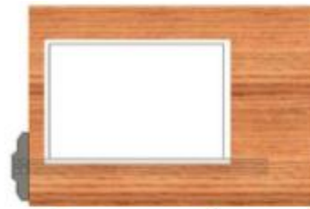
b) Place a T-square and move the paper until its lower edge lies close to the top edge of a T-square
