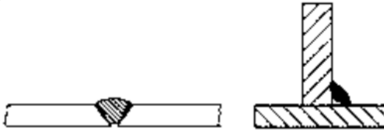
Figure: 4.5: Lack of Penetration
