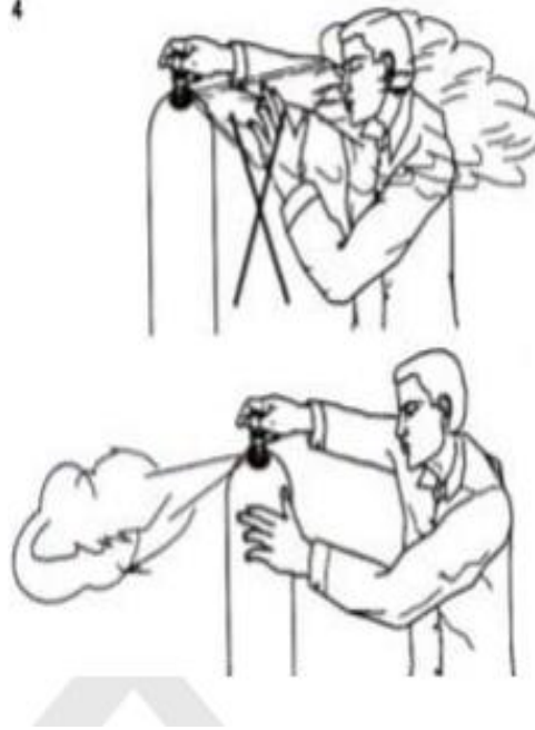
Figure.3.2. Safety concerning gas cylinders
