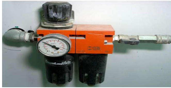
Fig.1.6 Devil Bliss DVFR-2 Filter Regulator, Coalescer
