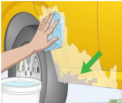
Fig: 1. Cleaning and Sanding the Surface
