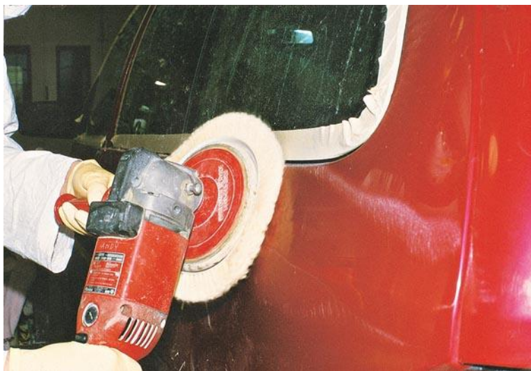
Figure 2.9. Polish the paint surface
