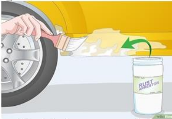
Fig : 3. Apply rust arrestor on the chipped area
