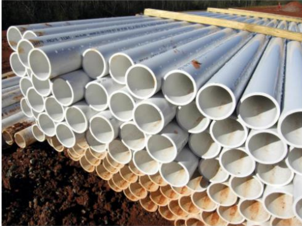
Fig 1.3 PVC pipes are commonly used to make perforated pipes.
