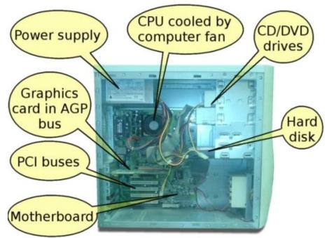
**Motherboard** is the body or mainframe of the computer, through which all other components interface. It is the central circuit board making up a complex electronic system. A motherboard provides the electrical connections by which the other components of the system communicate. The mother board includes many components such as: central processing unit (CPU), random access memory (RAM), firmware, and internal and external buses.
