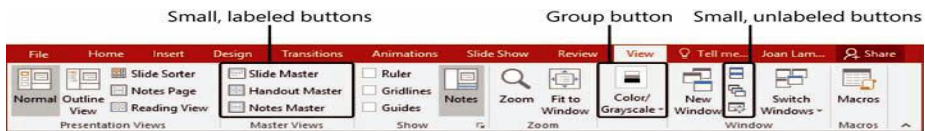
Fig2.9. When insufficient horizontal space is available, labels disappear and groups collapse under buttons
