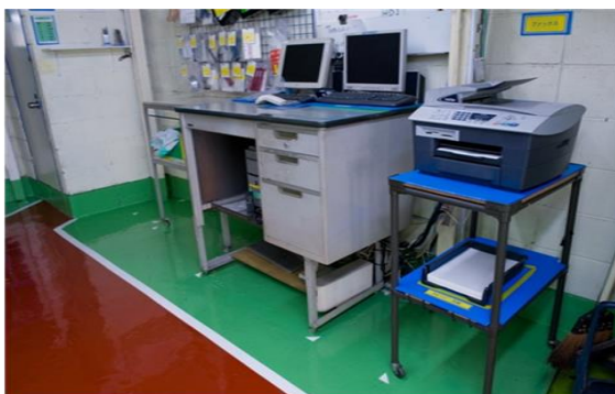
Fig 5.4. Indication of fixed position
