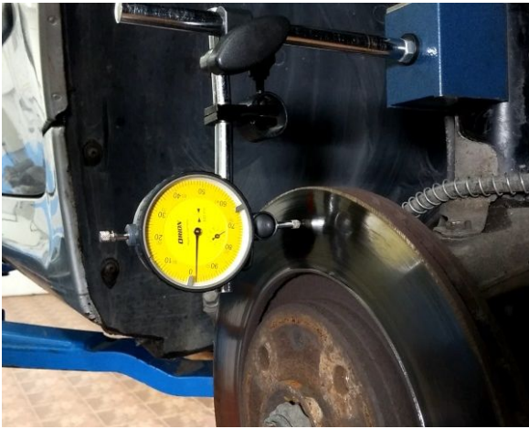
Fig.2.8. Checking brake disc flatness
