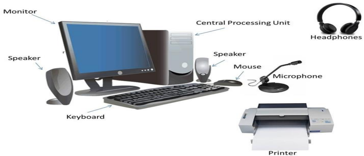
Figure1. 2 The typical set up of a personal computer
