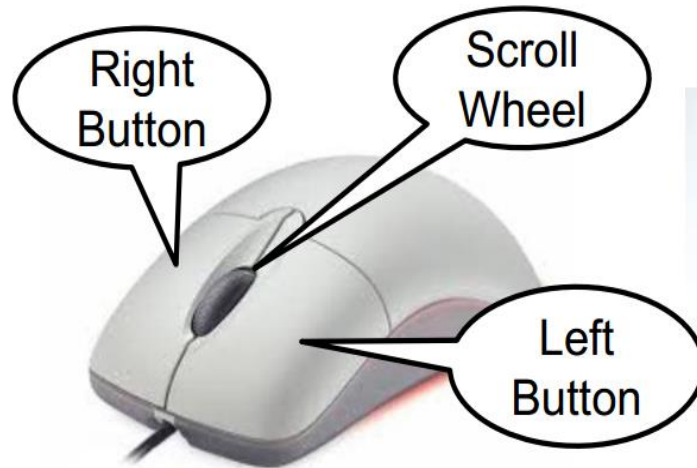
Figure1. 4 A mouse with two buttons and a scroll wheel
